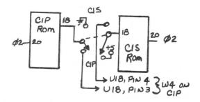
Wire all the pins in parallel with each ROM except for Pins 18 and 20. Both phase 2 clocks are at W6. Switch shown in old C1P ROM position.
