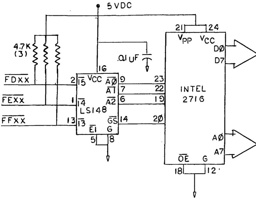
FIGURE 4: ALTERNATE DECODING FOR 2716 EPROM
