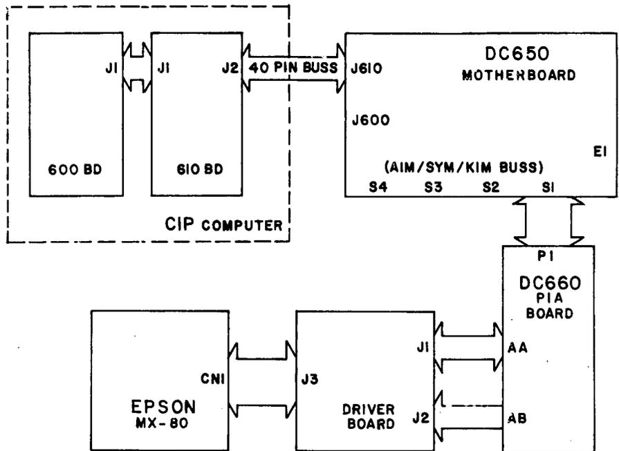
The DC660 Dual PIA board provides two PIAs (6820 or 6821). However, solder pads are also available to alter the chip's pin assignments to allow the use of Versatile Interface Adapters (VIAs - 6522s) in place of the PIAs. This chip is more powerful in what it does, but also costs more and is harder to program. (In either case, changing is easy, as the chips are socketed.)
