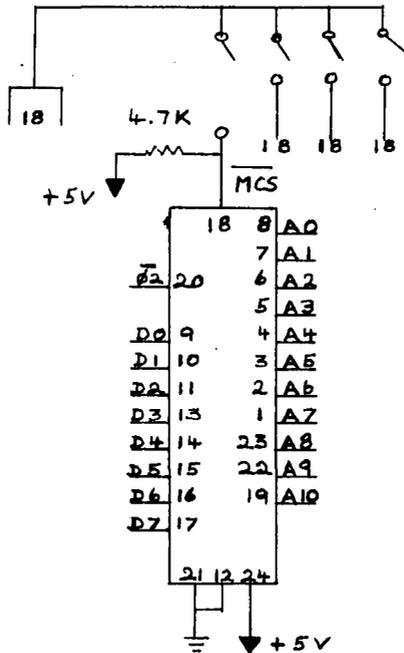
Wire up five 24 pin sockets in parallel as in drawing. Wire pin 8 to 8, Pin 7 to 7 and so on. Do this for all pins except Pin 18. Wire pin 18 of four sockets to a 4.7K ohm 1/4 watt resistor. Wire the other
