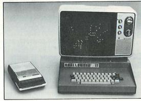
Complete with 8K BASIC-in-ROM, 4K RAM, a video board interface featuring 32 x 64 characters (lower case and graphic characters option available), an audio cassette interface, high quality keyboard, power supply and cooling fan all in one attractive case. Two of the four slots in the backplane are used, allowing some expansion. You need only to supply a video monitor for operation. For optional program storage, you'll want to add a cassette recorder.
